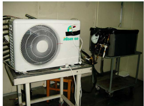
Fig. 18. Photograph of outdoor unit of hybrid air conditioner including storage unit.
