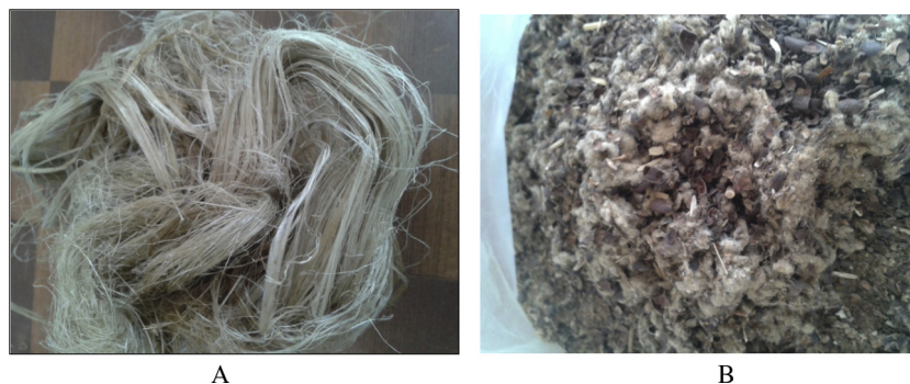
Figure 1 The photos of flax fibers (A) and cotton linters (B) before processing.
